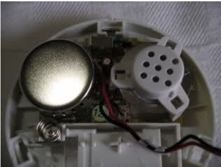
At the left side ionization chamber that protects access to the radioactive source
