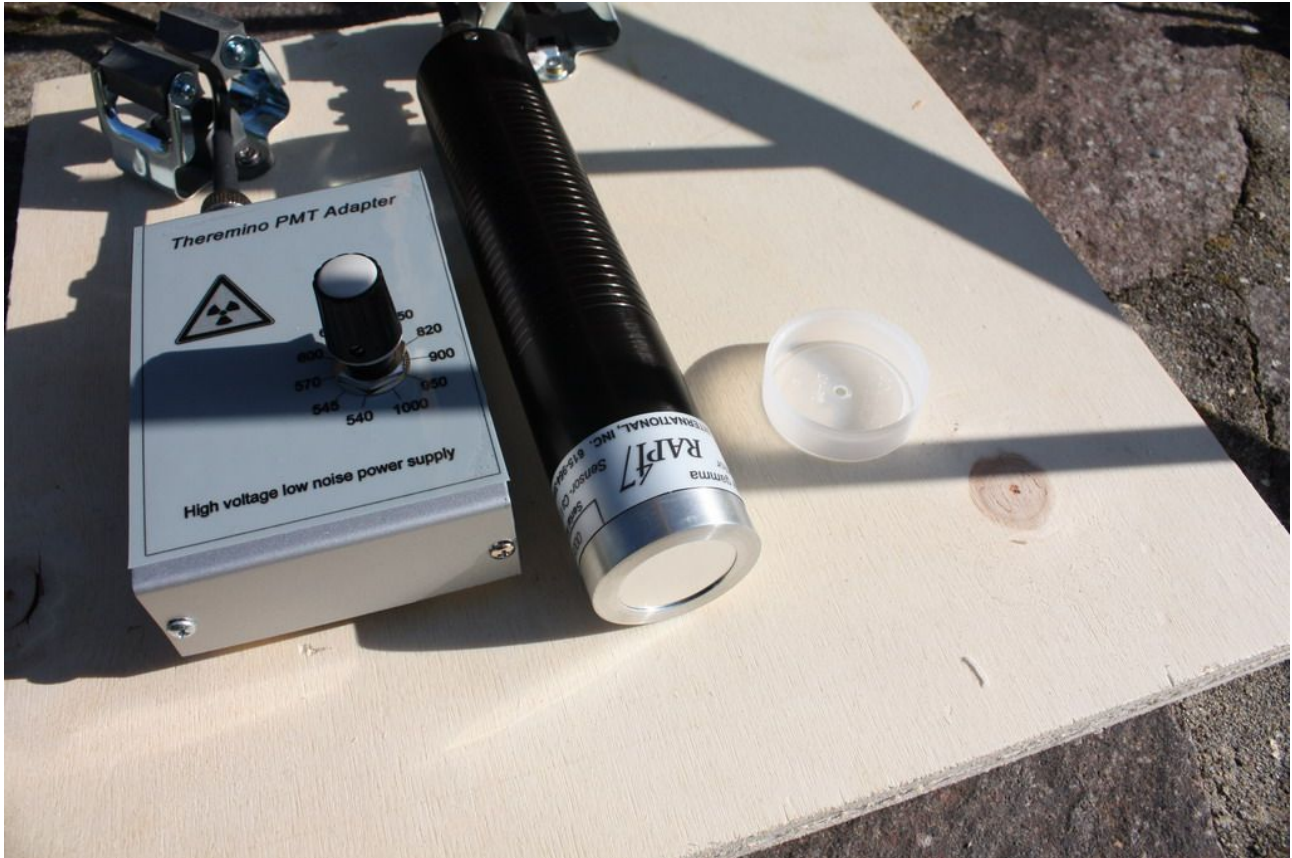
The probe RAP 47 with the Theremino PMT ADAPTER, low noise power supply
