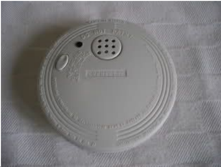
Ionization smoke detector
