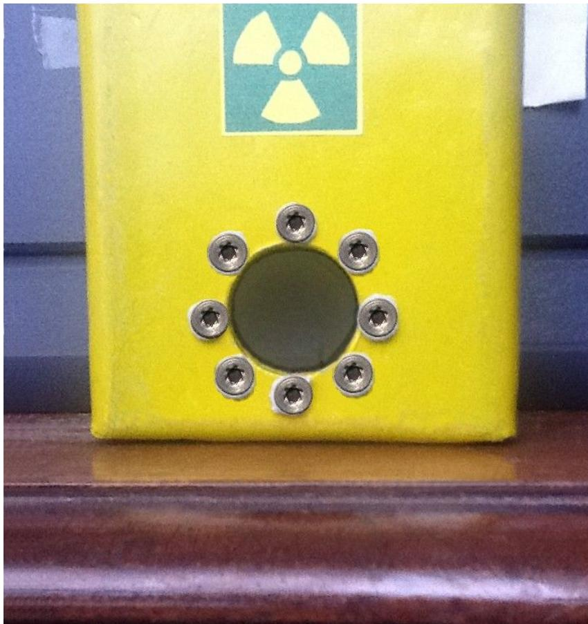
7 uCi of Am<sup>241</sup> (not 8 as in the above image) has been used, arranged around a hole in a lead plate, behind this hole a RAP47 25.4 x 1 mm probe was placed.
