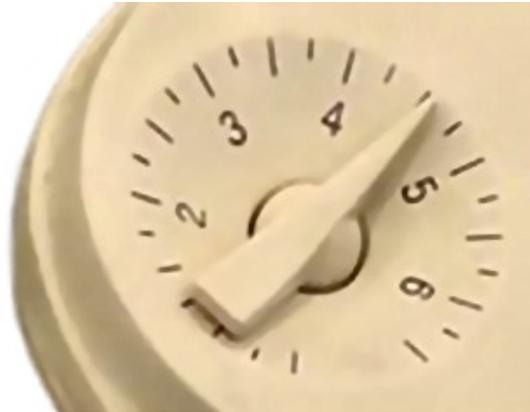
One of the known problems of the original instrument was the need to frequently reset the needle, due to the slow drift of the resistance of the subject during use. The Emotion-Meter application explores a new way to represent the resistance changes, by displaying the derivative.
