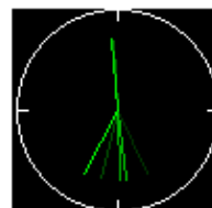
(f) AFC enabled, Fading History / Amplitude Display Mode Selected (2nd left click on scope)
