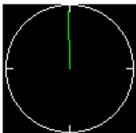
(b) The display with a normal psk31 signal. The vector flips between 0 and 6 o'clock
