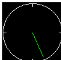
(d) AFC off and receive carrier set above the center of the received signal.
