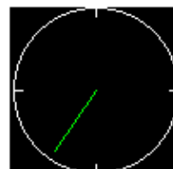
(c) AFC off and receive carrier set below the center of the received signal
