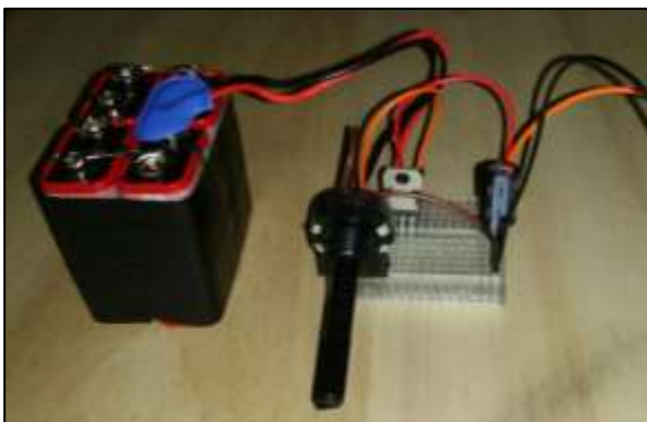
“Low noise” 30V power supply
