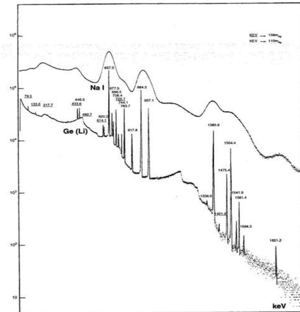
As we see the analysis of a gamma spectrum obtained with a scintillator may be difficult or even impossible to interpret. Here below we describe a method of deconvolution of the experimental data that can reconstruct the Gaussian shape of the photo peaks of a spectrum, making it suitable for a qualitative and quantitative analysis.
