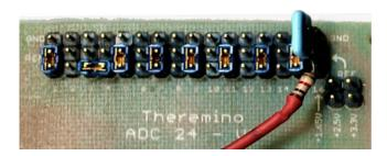
In the central bar (REF) it is injected the test signal, with the adapter visible in this image (the same adapter that is used for gain measurement).
