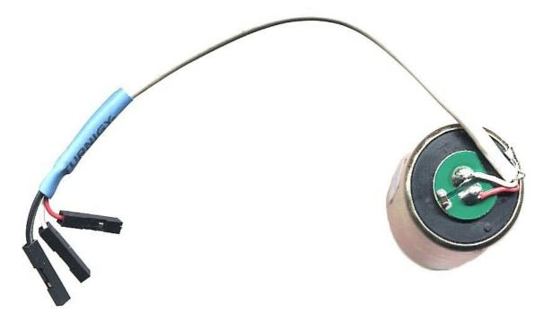
To solder the capacitor you remove two squares of green paint with a small, sharp screwdriver. In this way one can solder and desolder the capacitors without heating the wire anchoring zone, and thus without risking to move them or to dissolve their insulating sheath. Even if you use larger capacitors should the same solder at this point and not on the wires that are delicate and can easily deteriorate.
