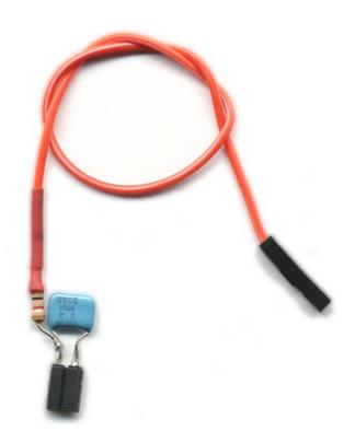
This adapter is a simple low-pass filter composed of a 1 kohm resistor (1/4 or 1/8 of a watt) and a 1 uF capacitor of any type. If the capacitor is electrolytic remember to connect the negative side to the ground (GND), that is the opposite side of the resistor.
