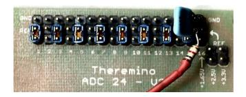
In the central bar (REF) it is injected the test signal, with the adapter visible in this image.
