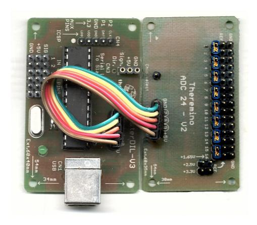
In this image we see the Adc24 equipped to measure the noise, with inputs closed with the jumpers.
