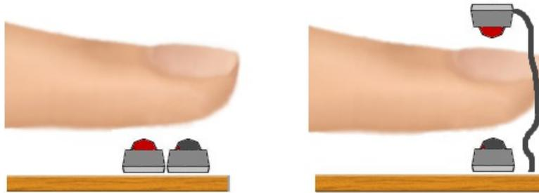
Until now there were only two types of sensors. Those with the LED and the sensor close together and those with LEDs above and below the sensor.
