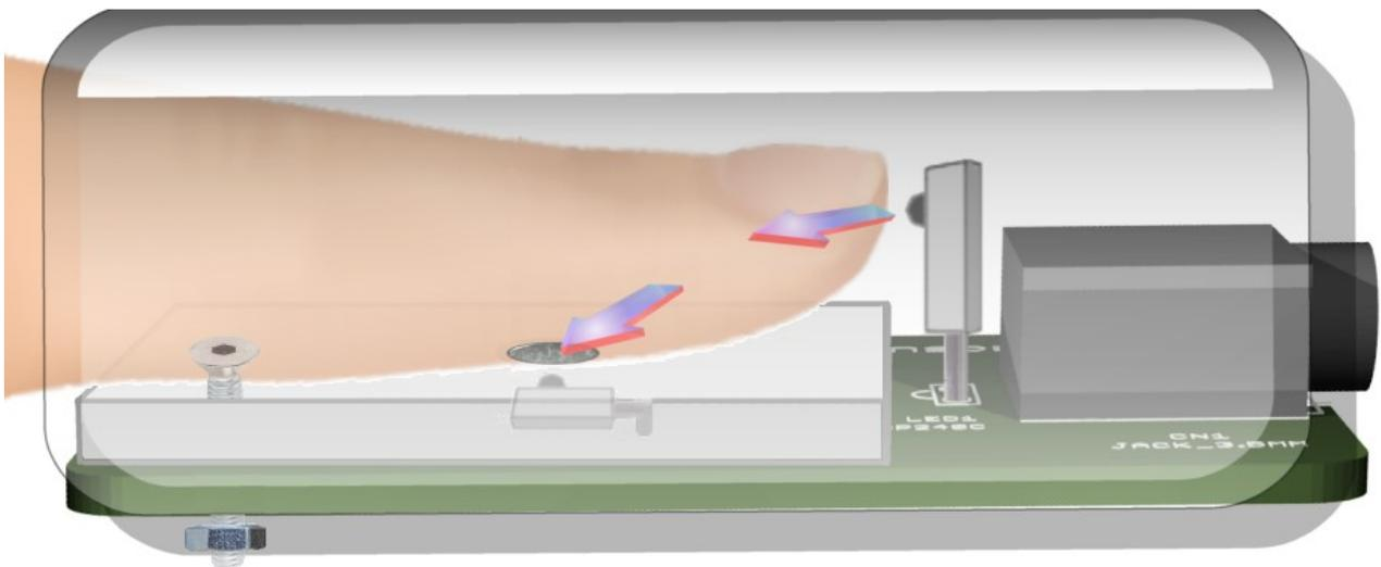
The screw will then be tucked inside. It will pass through the hole of the rectangle, the printed circuit board and finally released below through the cylinder bore. It puts a washer on the screw coming out, tightens the nut and the mounting is finished.
