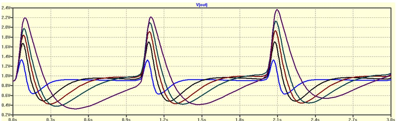
Here we see how the shape of the pulses with C1 and C3 which are worth 100 nF (blue), 220 nF (black), 330 nF (red), 470 nF (green) and 1 uF (purple).
