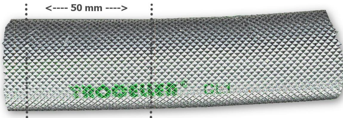
This is a piece of insulating coating for hot water pipes. you can find it in the hydraulic and thermo material retailers or by an installer of boilers or even by an hydraulic. They will give you a span without any problems or will sell a meter. It is a very cheap material.
