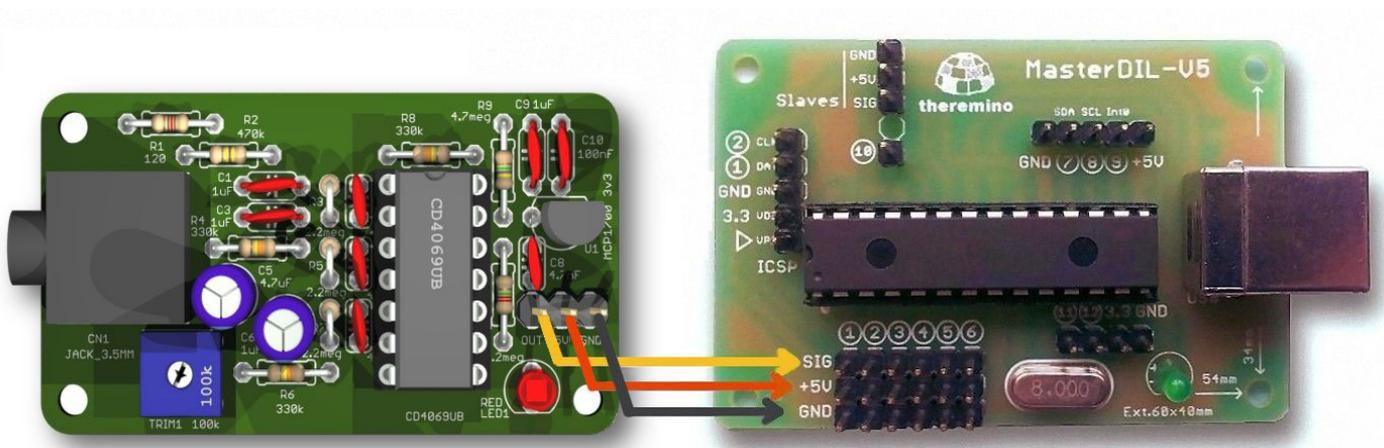
The connections between the amplifier and Theremino Master module are made with Dupont female female three-pin cable, as shown in this picture with the colors black, red and yellow. It is not necessary to use shielded cable for this connection.
