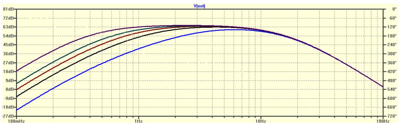
There **low cut-off frequency**, which is seen in the left side of the image part, it is determined by the value of C1 and C3 capacitors which can be from: 100 nF (blue curve), 220 nF (black curve), 330 nF (red curve), 470 nF (green curve) and 1 uF (purple curve).
