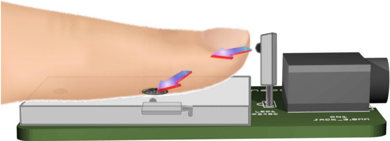
An infrared LED illuminates your finger from the tip. The infrared light passes through the skin and is more or less attenuated depending on the blood pressure. A photo-transistor (which is seen in transparency) collects light through a hole.
