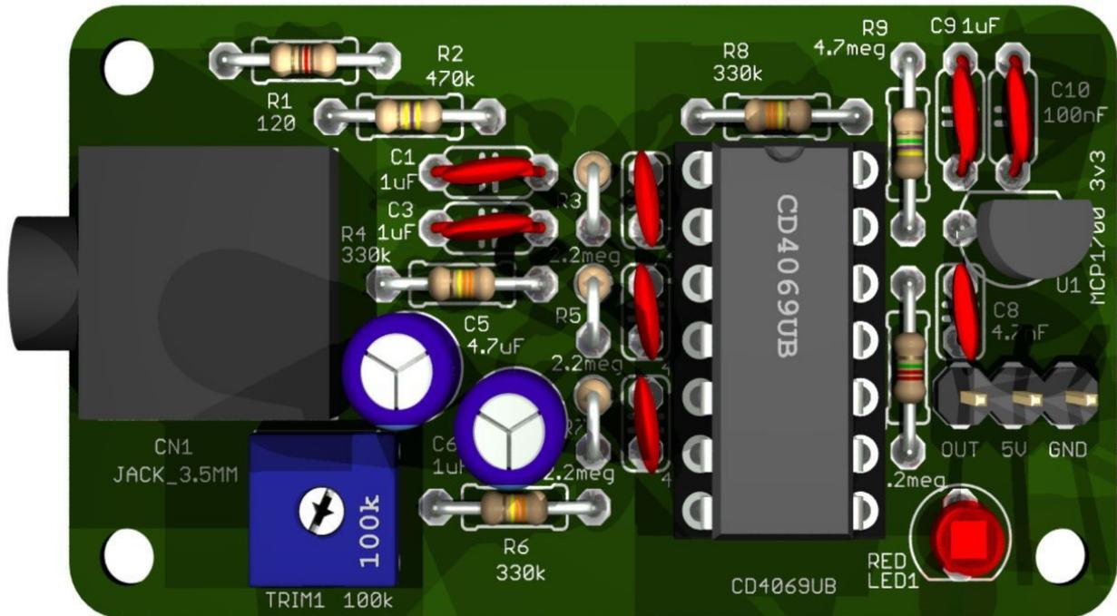
In this image it is to be noted the 1/8 watt resistors that allow a compact and orderly arrangement. In their place you can put those quarter-watt very tight bending.
