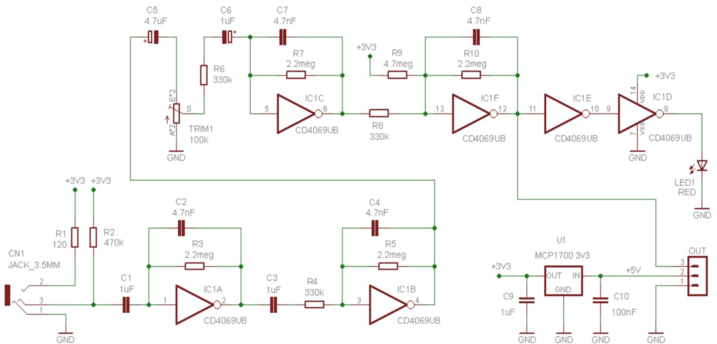
The resistor R1 sends a current of about 16 mA to the sensor LED.
