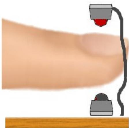
Benefits: There are not sensor glare problems. The light must necessarily pass through the finger.
