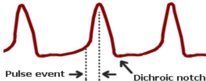
In practice, however, the waveforms that will be achieved will be a bit different from this, because we will use a high pass filter to eliminate the rocking due to the movements of the hand.
