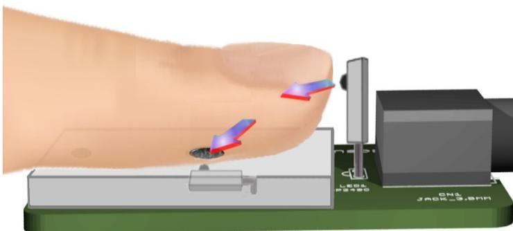
There is no glare sensor because the light necessarily passes through the finger. The light can only pass through the hole in the material that covers the sensor.
