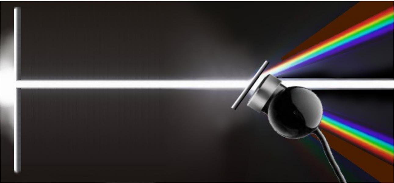
By placing a digital camera with a diffraction grating in front of the lens and **tilting with respect to the incident beam**, we obtain that the blue, violet and ultraviolet light components, hit the leftmost pixel and the red and infrared hit the pixel to the right. In this image, infrared light (invisible) is shown with a dark brown color. To detect the infrared is necessary to remove the camera built-in anti-infrared filter.
