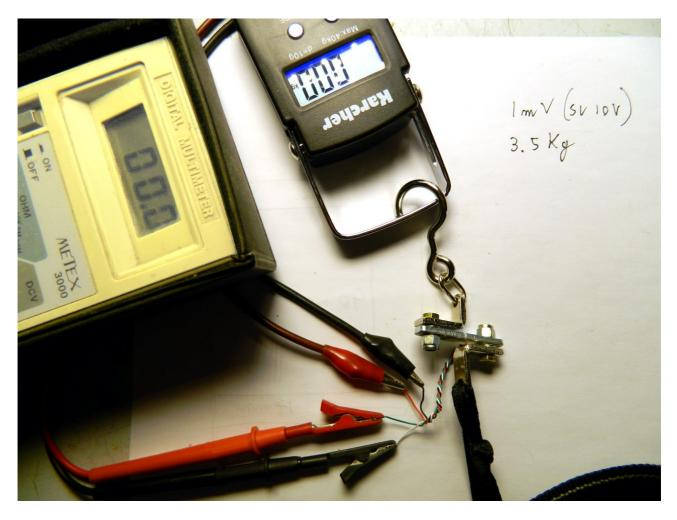
If you feed the cell with 10 volts you can obtain an output voltage of 1 mV with about 3.5 Kg.
