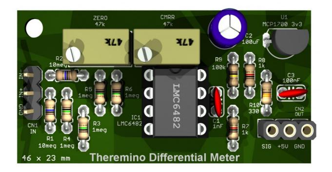
Reading a load cell with a generic module such as our Diff Meter, will not give an accuracy of +/- 10g.
