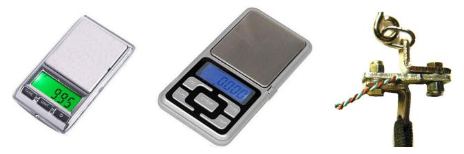
On the left a 0.01 to 100 gram scale, in the center a 0.1 to 500 grams, at the right a load cell from a "pull" 40 Kg Scale. All for sale on eBay for about 5 Euros, and all containing a load cell with four wires.
