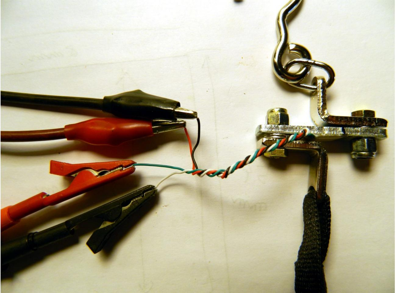
First of all prepare the wires, curled for extra strength and well skinned, to connect easily to a meter and to a power supply, during measurements.
