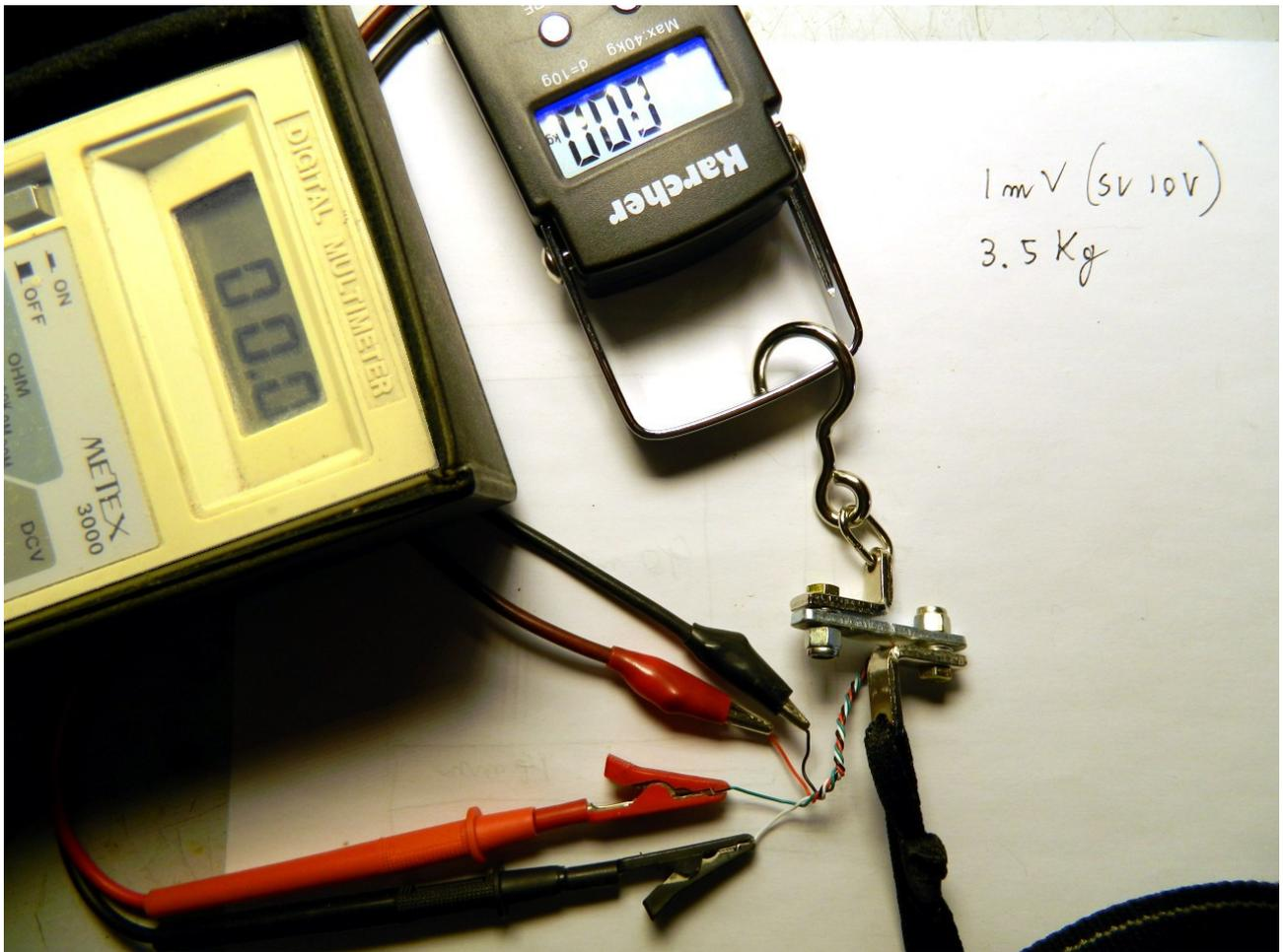
If you feed the cell with 10 volts you can obtain an output voltage of 1 mV with about 3.5 Kg.
