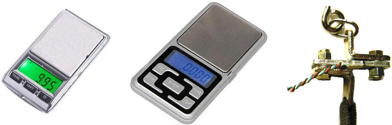
On the left a 0.01 to 100 gram scale, in the center a 0.1 to 500 grams, at the right a load cell from a "pull" 40 Kg Scale. All for sale on eBay for about 5 Euros, and all containing a load cell with four wires.
