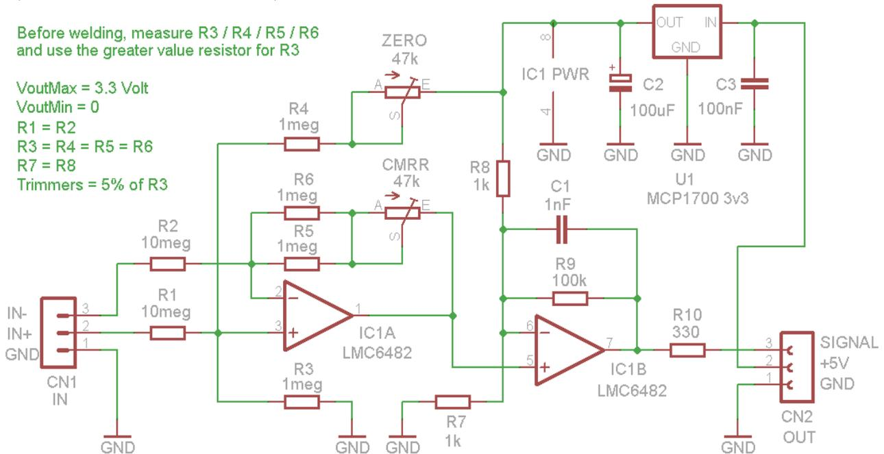
**The cell is to be connected in this way:**
