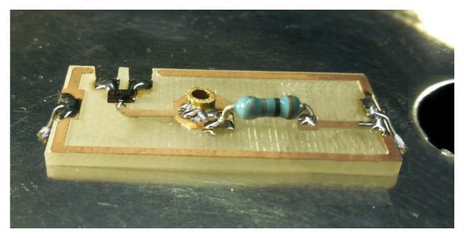
The FET module (like all other modules) is fixed by means of two bare wires welded to the base in tinplate or covered with adhesive copper tape. This module is then covered with a tin shield (tinned iron sheet) and the lid is welded on both sides.
