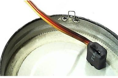
Furthermore (but we will see it better later), by covering the FET with a rectangular screen and the hole with a fine brass mesh, it is possible to make the open chamber work, with the electronics completely accessible, as seen in this image. And this is a great convenience when measuring components before closing the chamber.
