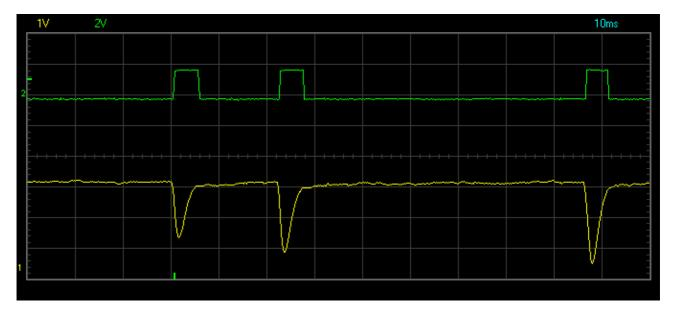
The yellow trace is the signal on TP3. In this point the pulses produced by the Radon are wide few milliseconds and fall of some volts, compared to the normal voltage that is approximately 3 Volts.
