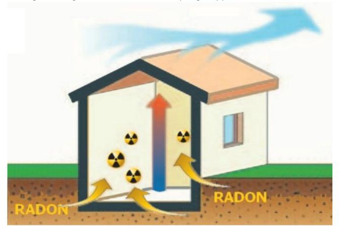
The main cause of the presence of radon in homes, is decreased pressure between the living areas and the ground. Decreased pressure is caused by wind and by differences in temperature, higher in winter when buildings are heated. The effects of this depression, results in the aspiration of air from the soil, with its radon content. The aspiration of radon is facilitated by openings such as chimneys, windows, skylights, as well as air extraction systems for the kitchen, bathroom, etc. ..
