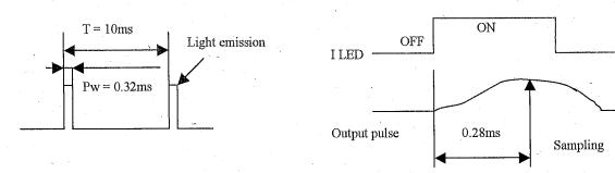
• Time required for the device to be ready to detect dust from when the system is turned on is less than 1 sec. Since GP2Y1010AU does not have peak hold circuit, the time is shorter compared with that of the conventional model (GP2U05/GP2U06), which have the peak hold circuit.
