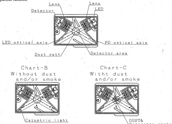
Light from the light emitter (Light Emitting Diode) is spotted with a lens and a slit as shown on the chart-A. Also for the light detector (Photodiode), a lens and a slit is positioned in front of it to cut disturbance light and to detect light reflection (when detecting dust) efficiently. Area where those two optical axis cross is detection area of the device.
