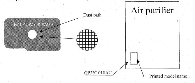
When dust collects inside the device and the sensor makes wrong output, please clean up by wiping up or by vacuum cleaner.
