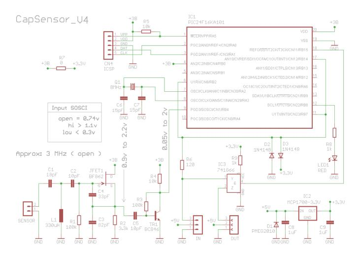
The connector Sensor and the components L1, C1, C2, C3, C4, C5, R1, R2, R3 and R4 form an oscillator with a very low noise, almost a front-end for radio receiver, and compose, together with the PIC, a 24-bit ADC being able to follow infinitesimal changes in capacitance, with stability of one part in two million.
