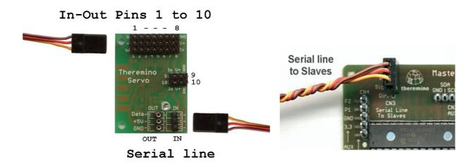
The serial line from the Master must be connected to the "IN" of the first "Slave"
