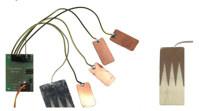
They can be constructed easily by cutting, even by hand, from a sheet of single face copper **Vetronite**.
