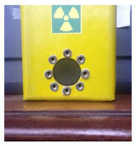
7 uCi of Am241 (not 8 as in the above image) has been used, arranged around a hole in a lead plate, behind this hole a RAP47 25.4 x 1 mm probe was placed.
