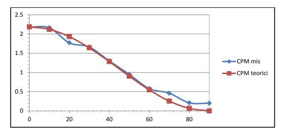
The detector measures values less than the theoretical ones due to the fact that the detection angle is limited (see construction scheme), for this reason, the theoretical values have been normalized so as to match the maximum.
