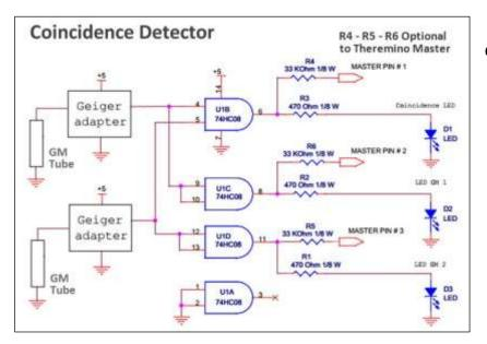
**Coincidence detector circuit**
