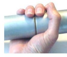
This electrode can be easily holding with one hand, placing the isolated junction in the center of the palm of the hand.
