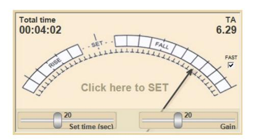
The continuous zeroing produced by the derivative of the signal and an automatic autorange, make it much easier to use the instrument also for solo use.
