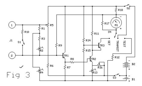
This is the original scheme, the Hubbard patent. There are five trimmer to adjust and uses germanium transistors which change the characteristics just looking at them. Despite to you adjust well, it will always be very inaccurate.
