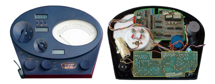
In the original equipment, and also in the Theremino Emotion-Meter, the resistance is measured by means of a weak electric current, in the order of tens of microamperes. A completely harmless and not perceptible current.
