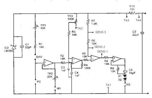
This is a more recent scheme, much better, but with three calibration points, therefore difficult to adjust accurately and fairly sensitive to changes caused by the component's aging.
