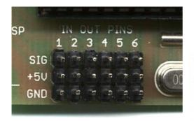
Sensors and actuators are connected to the "IN OUT PINS" with standard cables (male to female extensions)
