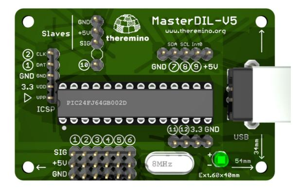
The Master module has to be connected to a USB port (usb1, usb2 or usb3), and provides twelve Generic InOut Pins. Earlier Master versions had 6 Pin (versions 1 and 2), or 10 Pin (Version 3). So to know the Master version, just observe how many Pins are listed.
