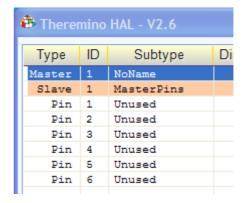
To turn on the LEDS you must configure their "Pins" as DIG\_OUT, Pwm\_8 or Pwm\_16
