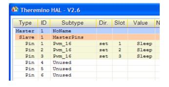
The "Sleep" changes to a number from 0 to 1000, and the brightness of the LED of that line is adjusted from minimum to maximum. For better adjustment in the lower area, set "Logarithmic response" to all LEDS.
