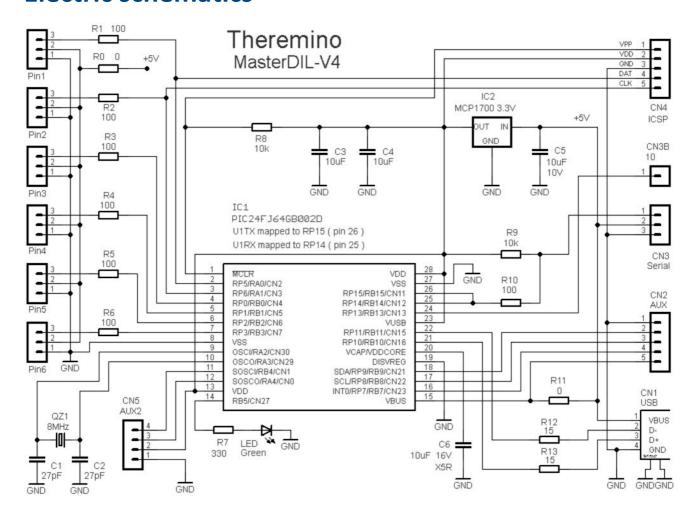
The six connectors Pin1 to Pin6, with protection resistors R1 to R6, provide six InOut generic pins, configurable to connect all kinds of sensors and actuators with the standard: GND / +5 V / Signal
