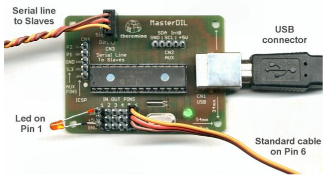
Here you can see an LED connected to "Pin 1" ...
