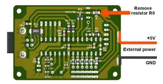
Unsolder (or break with the clippers) the resistor RO and solder red and black wires to bring the +5 Volt from an external power supply.
