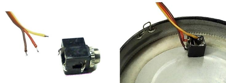
Shorten the terminals of female jack with the clippers, stagnarli well and finally solder the three wires to the socket. Check that the brown wire is connected to the base, the red wire to the central and the yellow wire to the tip of the jack. If necessary, insert a jack and check with the tester.
