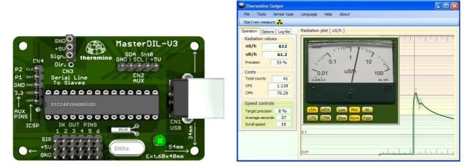
Normally you use a module Theremino\_Master that provides the power for the ion chamber and sends counts to Theremino\_Geiger software, via USB. Only one Master can power up to six ion chembers, with links to hundreds of meters long and collect all of the data. Some of these could be replaced with six chambers probes Geiger rays for Alpha, Beta and Gamma or with environmental sensors, to measure, for example, the mm of rainfall, temperature and humidity.
