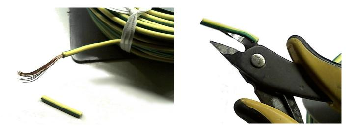
Peel a few inches of wire for electrics and cut it to length with the clippers.
