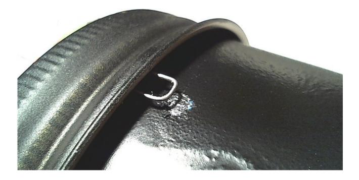
Before doing the electrical tests, you must connect both the bottom cover, the two top covers. We recommend that you solder the treble of the first top cover and saldarne at least one for each of the other two.
