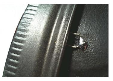
If you miss part of the shield also tests on noise TP3 with the oscilloscope will not be significant and you will see a strong ripple at mains frequency (20 msec cycle equal to 50Hz).
