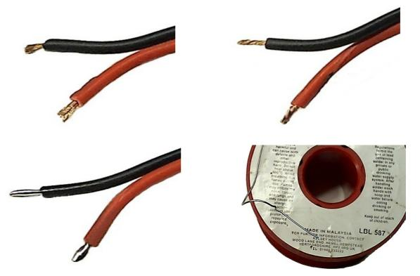
Before making connections all the wires must be stripped, tinned and curled one by one. The pond must be leaded With flux and thin (half a millimeter). Even the terminals of the circuit boards must be prepared, stagnandoli with a nice shiny ball.
