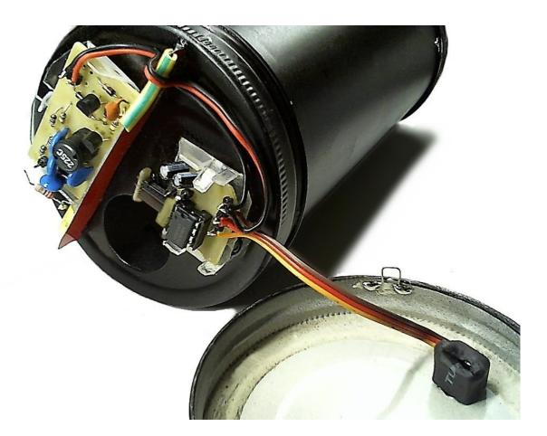
In this picture you see the new simplified wiring. In early versions of the modules were interconnected with connectors, but it was difficult to make them fit in the small space available.
