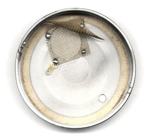
The dust filters are two, on the outside covers holes. Here is a simple and effective way to secure them. A second square of brass mesh is welded on one corner. On the opposite corner is welded a metal plate or a piece of stiff wire. In this way, the filter can be taken on and off easily. Place the filter being careful to cover well the hole and fold the plate to secure it.
