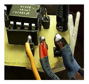
When the wires are two (or three) it is good to keep them together with a piece of the sheath. This makes it much easier to weld and unbrazed terminals of printed circuit boards.
