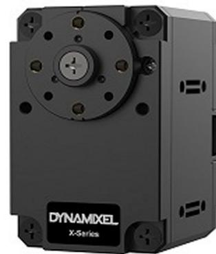
Some Dynamixel motors can be controlled in a range of +/- 256 rpm, while currently the FeeTechs (**Note 1**) they have a smaller range, of only +/- 7.5 turns.
