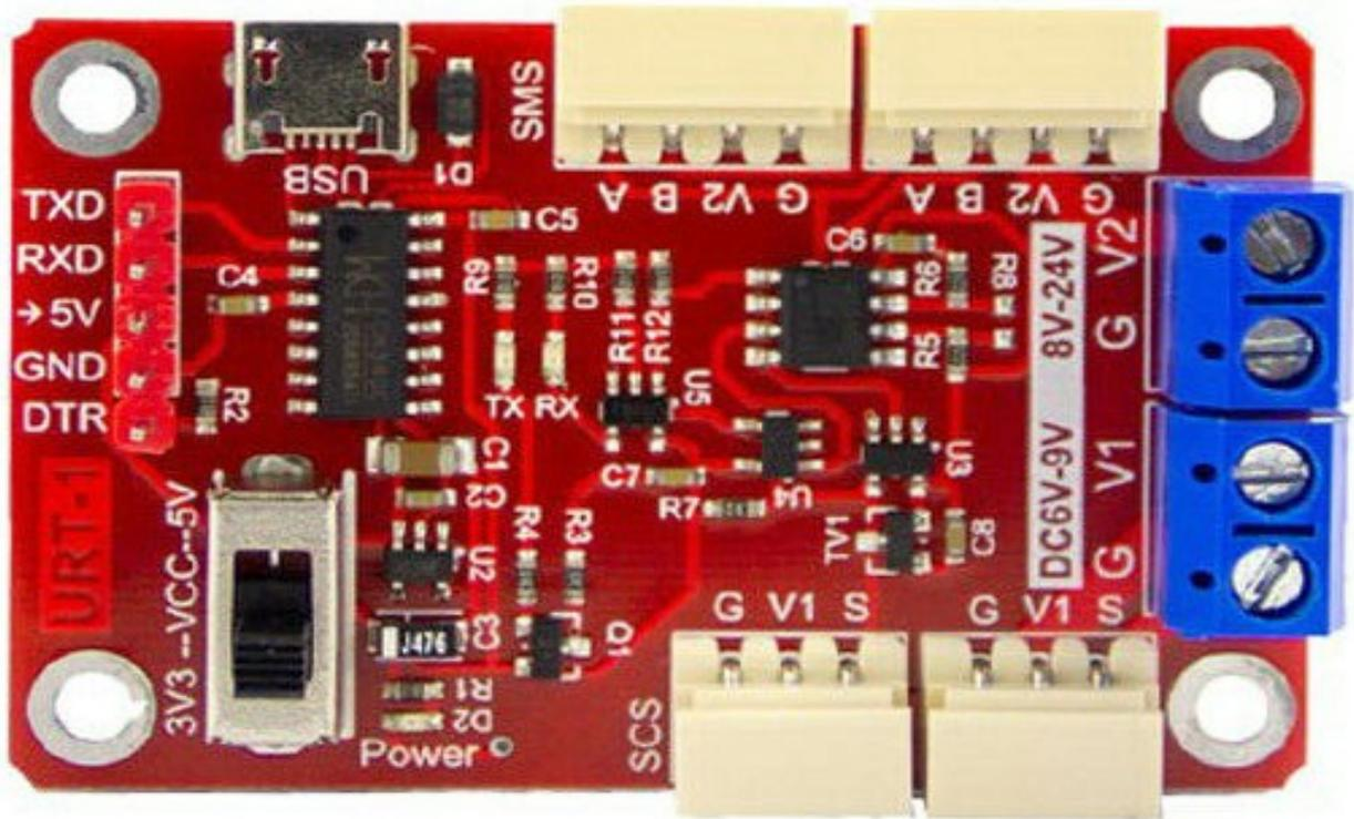
This module could also be connected to an Arduino by means of a serial link.
