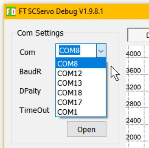
In this case the port was COM8 but if the list of ports remains the same, both with the USB cable and without the USB cable, then you will have to install the CH340 driver and then repeat the instructions on this page.
