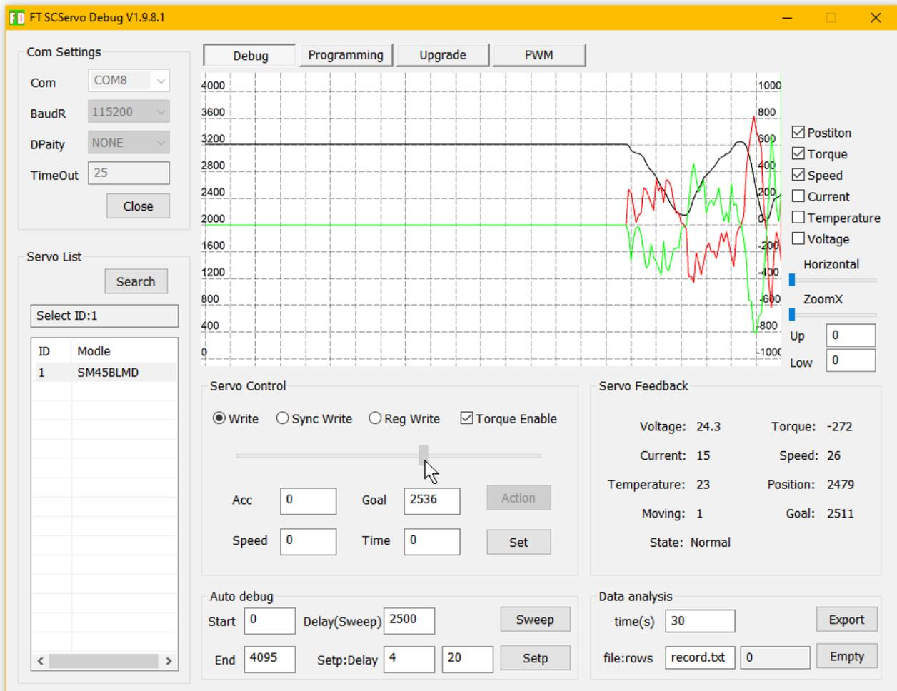
To move the motor it is necessary that its name (in this case SM45BLMD) is selected in the white list on the left. Click with the mouse on the name.
