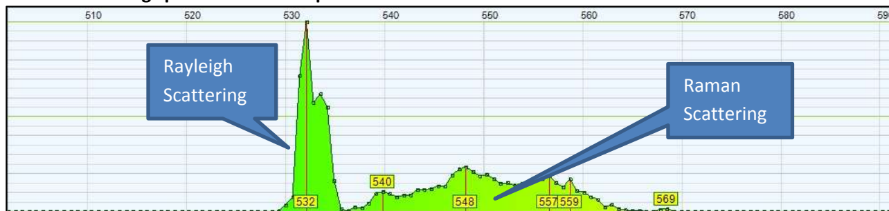
Raman scattering spectrum of chlorophyll alcoholic solution - Excitation 532nm laser
