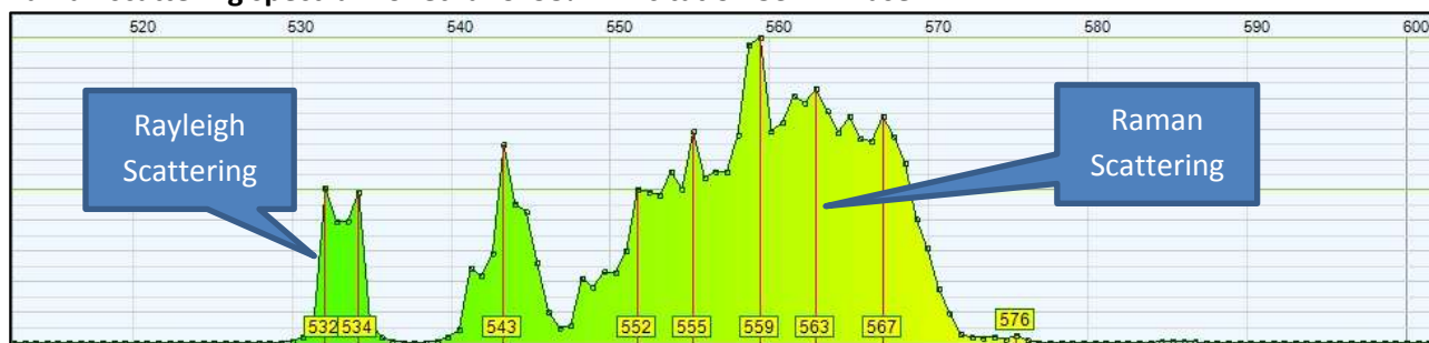
Raman scattering spectrum of ethanol 95% - Excitation 532nm laser
