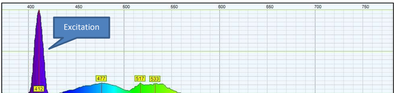
Fluorescence spectrum of halogen inner bulb excited by UV emission
