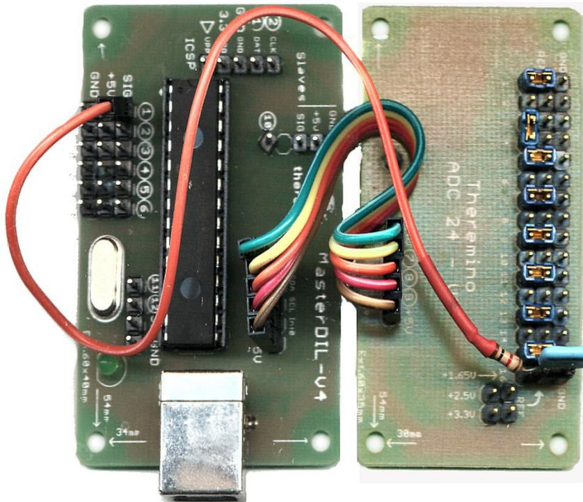
In this image we see the Adc24 equipped to measure the intermodulation between channels. The second input has an horizontal jumper, as in the noise measurements. While all other inputs is injected the strong signal coming from the PWM output, Pin 1 of the Master.
