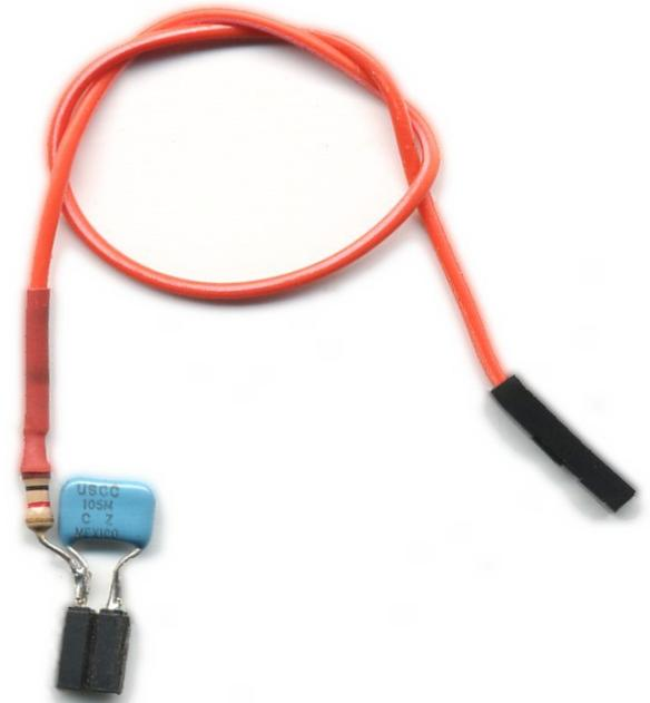
This adapter is a simple low-pass filter composed of a 1 kohm resistor (1/4 or 1/8 of a watt) and a 1 uF capacitor of any type. If the capacitor is electrolytic remember to connect the negative side to the ground (GND), that is the opposite side of the resistor.
