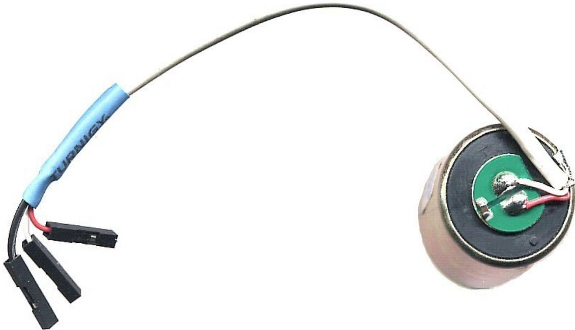
To solder the capacitor you remove two squares of green paint with a small, sharp screwdriver. In this way one can solder and desolder the capacitors without heating the wire anchoring zone, and thus without risking to move them or to dissolve their insulating sheath. Even if you use larger capacitors should the same solder at this point and not on the wires that are delicate and can easily deteriorate.
