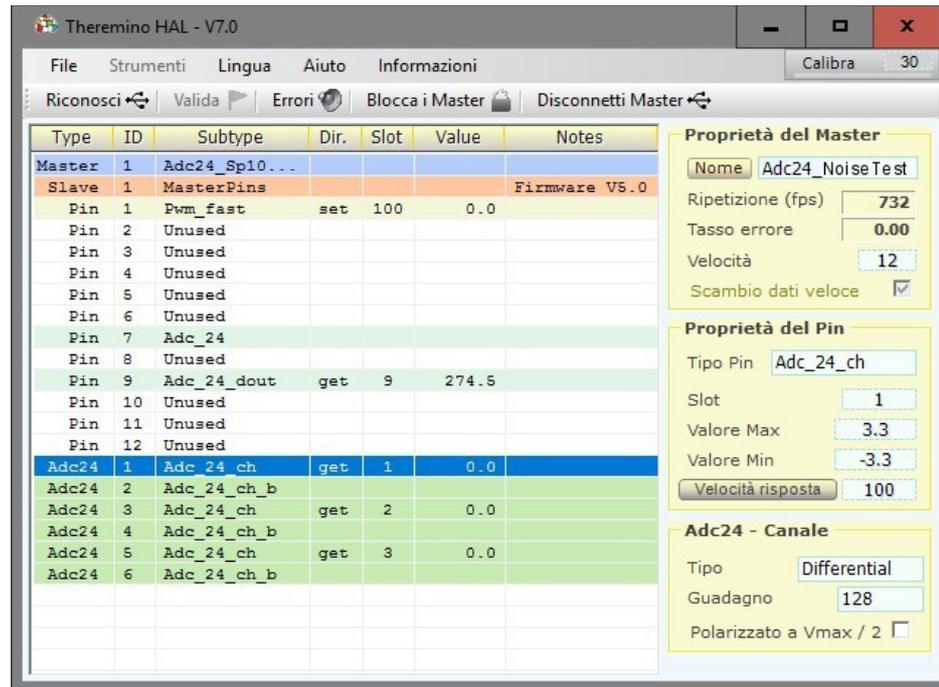
On the AdcTester application press the "Load configuration" button and load the "Adc24\_NoiseTest" file.
