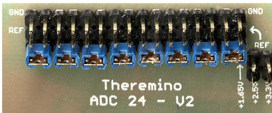
In place of the jumpers, you could connect shielded or simply twisted cables.
