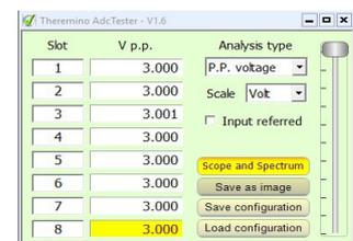
**Save configuration** - Save all configuration parameters, including even the oscilloscope and the spectrum analyzer settings. It is recommended not to edit files "Adc24\_GainTest.txt", "Adc24\_NoiseTest.txt" and "Adc24\_ImodTest", but to give a personal name to the file. **(Note 1)**
