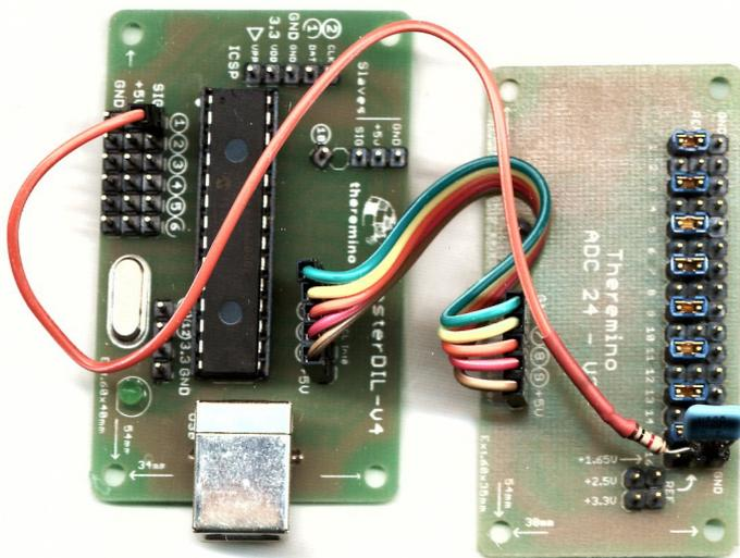
In this image we see the Adc24 prepared to measure the inputs gain.
