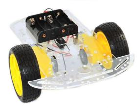
Vehicles with two wheels and a freewheel are the most difficult to control. To make them go straight you need to keep track of the speed of the motors with perforated discs and optical sensors.
