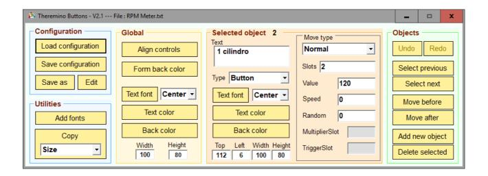
With this window commands you change the controls, the display text, the colors and the readwrite properties of the Slot signals. Then you dispose the controls and create new controls and delete them.
