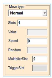
**Important**: If you set the "-1" value to "Multiplier Slot", or if the slots indicated by "Multiplier Slot" contain zero, then the text box displays the text that was written in the "Text" property.
