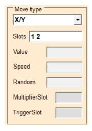
The type X/Y acts on two axes independent between them. In the Slots box you set up two numbers to indicate the slot on which to write the X and the Y values. You can therefore control a pointing device, for example a camera, or drive a vehicle with steering wheels.
