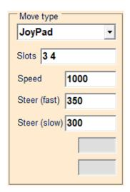
All Joy modes (no XY) They are for vehicles with two motors connected to left and right wheels or tracks. Giving more power to the right motor you turn to the left and vice versa. In the "Slots" box you specify the Slots of the drivers for the left and right motors.
