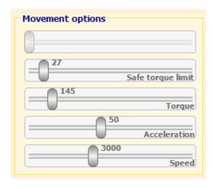
The first slider at the top, which is disabled here, is for limiting the pair in "Collaborative" mode.
