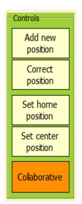
Pressing Add new position a line is added to the sequence MoveTo with the current position of all motors.
