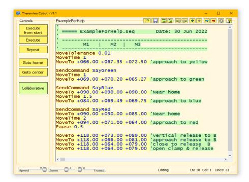
This application contains the necessary to move a Cobot, i.e. a robotic arm or any other mechanism designed to collaborate with humans.
