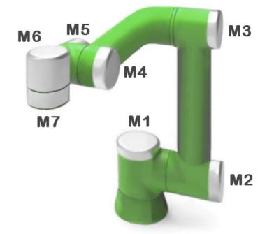
The End Effector is an interchangeable tool which could be a pliers, a screwdriver, a suction cup or other tools for soldering, gluing, etc.
