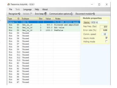
If the system doesn't recognize the USB port, the first line where it is inserted "Module", turns red, indicating "DISCONNECTED" and the window "Module properties" turns orange. In this case, click on "Recognize" and if u have working HW connected, everything should be fine.
