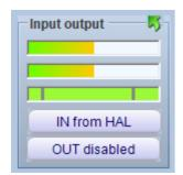
In from HAL, is used if sensors or ECG devices are connected, having output signals in Volts (0-10) or in mA (4-20), through our MASTER modules. When using this input, HAL also appears in the application bar, near the Theremino ECG icon
