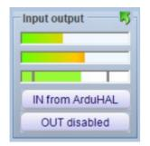
In from ArduHAL, allows you to connect devices with Arduino firmware, such as our OCG finger sensors, to the PC via USB port.
