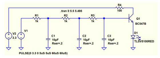
This scheme is the LED driver. The input signal is coming from a FastPwm Pin set to 20 KHz. After the LED there is a photo-resistor (less than 1 k at 100 lux) that replaces the potentiometer.
