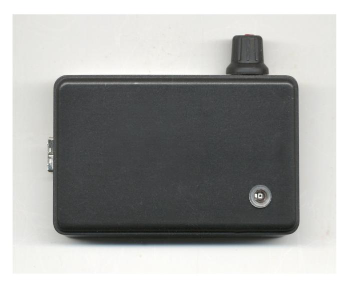
On the left you see the USB plug, at the top the knob adjustment potentiometer and at the bottom right the sensor (a TEPT5700 photo-transistor which has an almost flat top).
