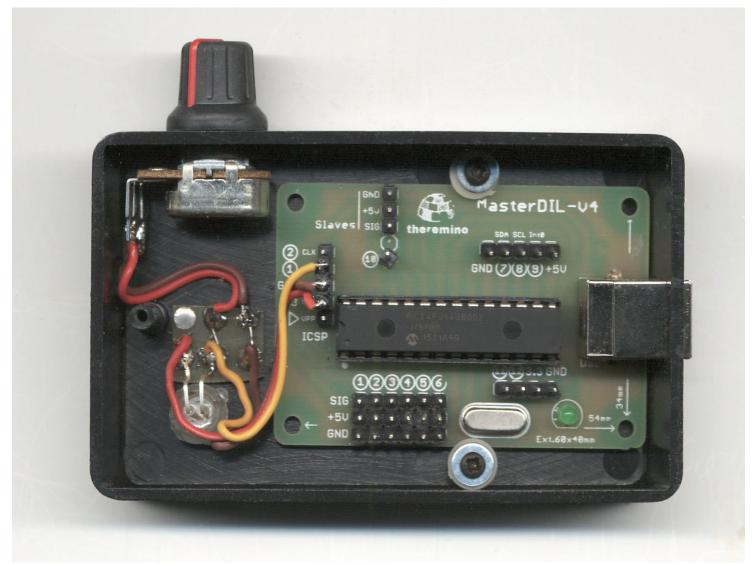
The brown and red wires are connected to potentiometer side and central. If you connect the wrong side the potentiometer will work inverted (decrease the signal by turning it clockwise) if so, just weld the wire on the opposite side.
