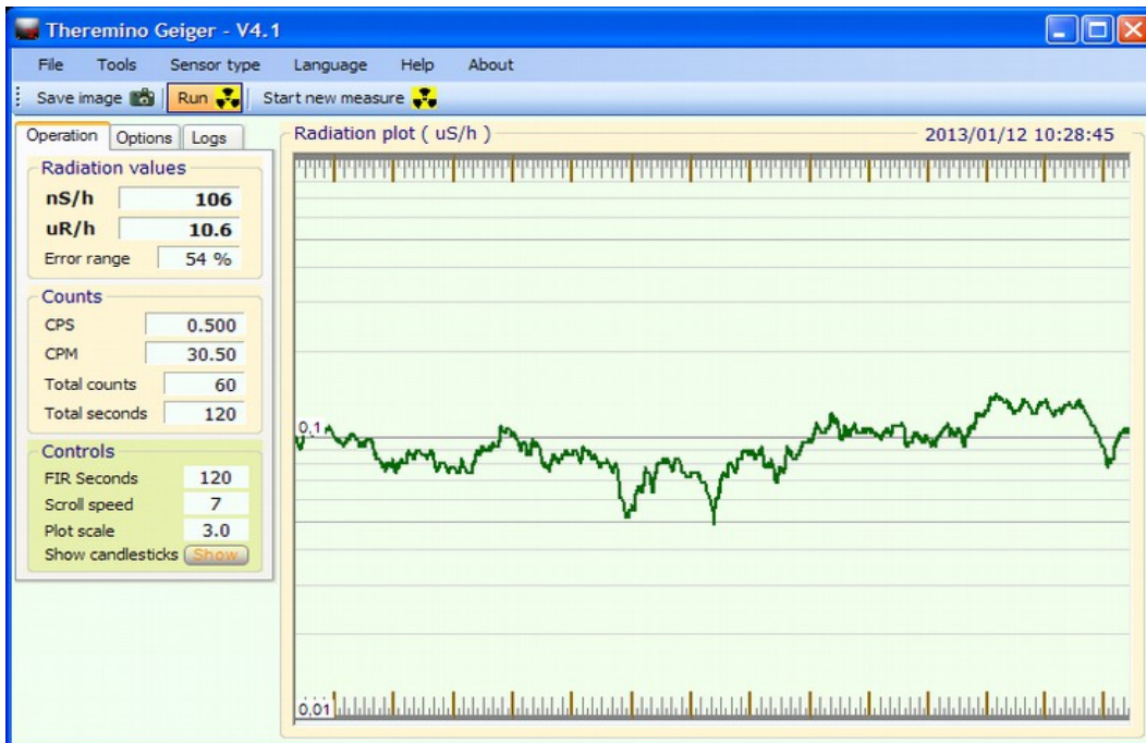
Fund environment with a tube SBM-20 and FIR filter set to 120 seconds
