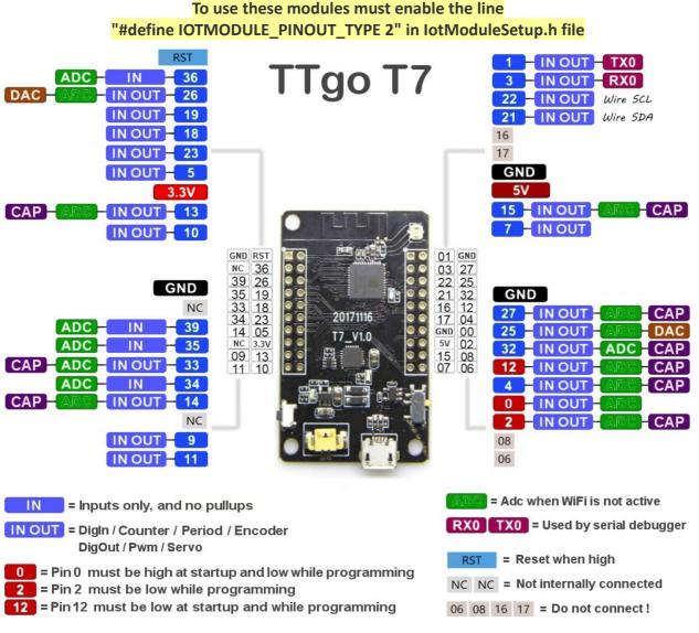
Leave Pins 0, 2 and 12 open, or use them as output only, to control high impedance devices Pins 2 and 12 could be input-pull-up, connected to GND with a button or an open collector
