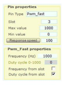
The minimum frequency that can be generated is 0.02 Hz and the maximum is about 40 MHz. The Duty Cycle goes from zero (always low output signal) up to 100% (always high output signal).
