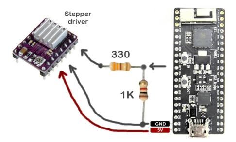
The two resistors of this image must be repeated for each STEP and DIR wire that goes from the IOT module to the Stepper Motor drivers.
