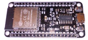
We have found that to make operating this model of modules, you must connect the Pin "0" to 3.3 volts through a 1k resistor (if you connect it directly no longer able to program). Moreover this model has no LEDS and has the WiFi antenna works very badly, it works only near to the Access Point.
