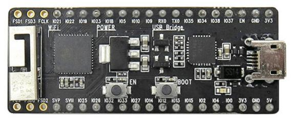
This is the model that we prefer ESP32, it communicate faster than the others, has a larger number of Pin and the pin layout is better.
