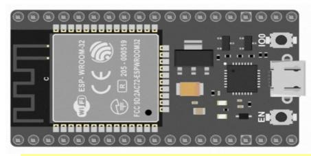
To use these modules you must enable the line "#define IOTMODULE\_PINOUT\_TYPE 1" in the "lotModuleSetup.h" file This ESP32 model is to be used as second choice. To use these modules you must enable the line "#define IOTMODULE\_PINOUT\_TYPE 0" in the "lotModuleSetup.h" file
