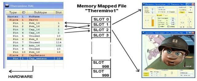
In this only the HAL writes in the Slots, but in reality all the components of the system can both read and write in any of the Slots, even if already used by others.
