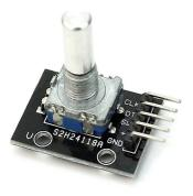
There are Encoders like small pots (the best known are the KY-040 of this image). These models are mechanical and provide 18, 20 or 24 pulses per revolution depending on the manufacturer. The firmware obtains from these pulses 72, 80 or 96 angular positions for each revolution, if adjusted in the software mode (x2), or 36, 40 or 48, if adjusted in hardware mode (x4).
