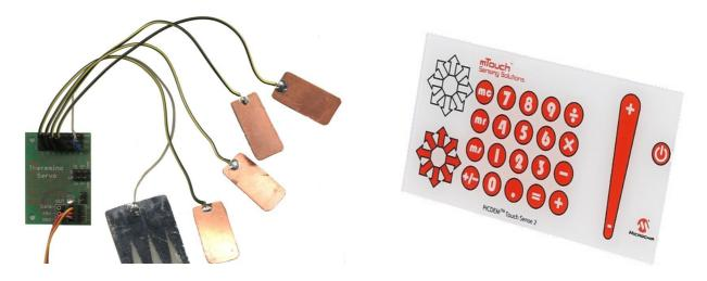
Capacitive keys cannot replace CapSensor modules, the first work only at short distances (from a few millimeters to a few centimeters), while CapSensors work up to distances of several meters, and can be adjusted for an almost perfectly linear response. The capacitive keys on the other hand are much cheaper and are better suited to arrange keyboards with many keys.
