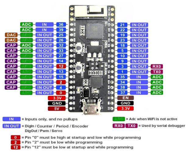
Leave Pins 0, 2 and 12 open, or use them as output only, to control high impedance devices Pins 2 and 12 could be input-pull-up, connected to GND with a button or an open collector
