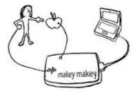
keys, you can connect more Makey Makey in chain, but at the end, all keys are sent to the keyboard that manages just a maximum of six: <u>www.makeymakey.com/faq</u> Finally, the Makey Makey keys have only on/off operation, without intermediate adjustments and do not feel keys pressing speed (Velocity).
