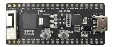
The IotModule (ESP32) works with 5 volts and communicate via WiFi with an Access Point, or directly with the PC equipped with a WiFi module that supports Mobile HotSpot function. For example, a notebook or a recent Tablet with Windows 10.
