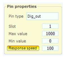
"Slot" indicates where to write or read data. The slots are a thousand, numbered from 0 to 999, and can be read or written by all the Pin and all the Theremino system applications.
