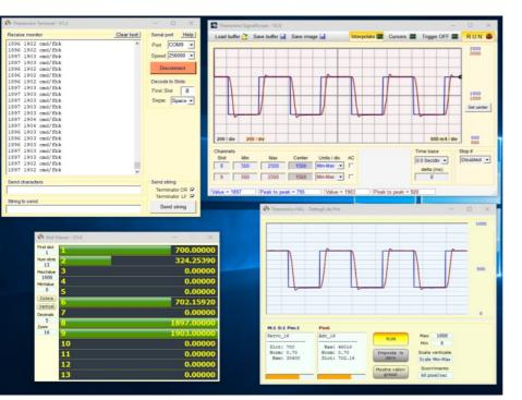
In the firmware, the values of the variables to be followed are sent to the serial port and the <u>Terminal</u> <u>application</u> interprets the values and sends them to the Slots.
