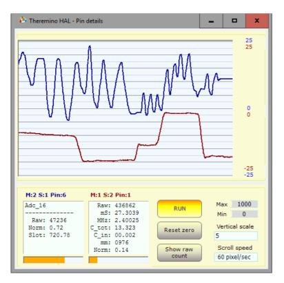
With a double-click on a active Pin line, this instrument is opened. To display two signals click on the first Pin then on the second Pin, with a single click.
