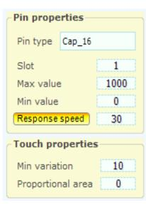
This type of Pin allows you to read simple buttons like with a Makey Makey (<u>http://vimeo.com/60307041#</u>) but with superior performance. (the keys are not resistive but capacitive and therefore can be adjusted to work even just by touching them, without contact, through an insulator and without an earth connection additional wire)
