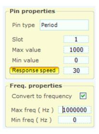
The Pin programmed as Period or Period\_pu can be transformed from counter to frequency meter.
