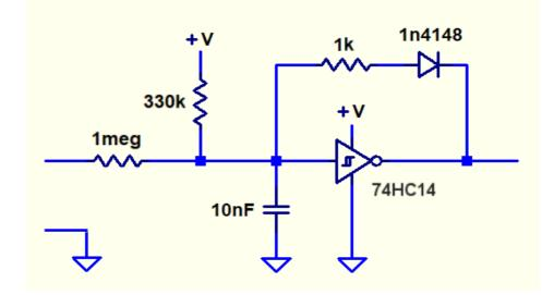
With this circuit every digital input can become an ADC. You will then have up to eight ADCs on a NetModule, or transform to ADC the Pins 7 to 12 of a Master.
