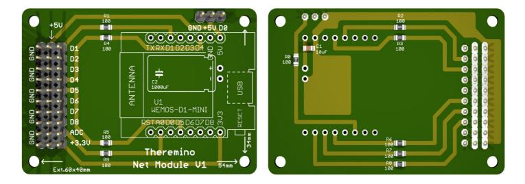
On the left are the input and output connectors. For convenience all connectors bear the mass, the 5 volts and the signal. The last connector in the bottom instead of the signal provides the 3.3 volts stabilized voltage, useful for some sensors.
