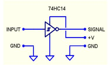
In some cases this measure may not be necessary, but it is for sure if you have input signals with slow edges (longer than 1 uS) and if the pin is configured as Period or Counter input.
