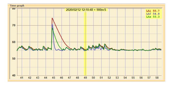
The levels displayed are maximum levels calculated on intervals equal to 1/8 s. The profile with the greatest variability is the one with a FAST time constant (8 dB), while the one with the least variability is the SLOW one (3 dB). The IMPULSE profile is systematically maintained above the FAST and SLOW profiles, denoting the impulsive characteristic of the noise emitted by the machine.
