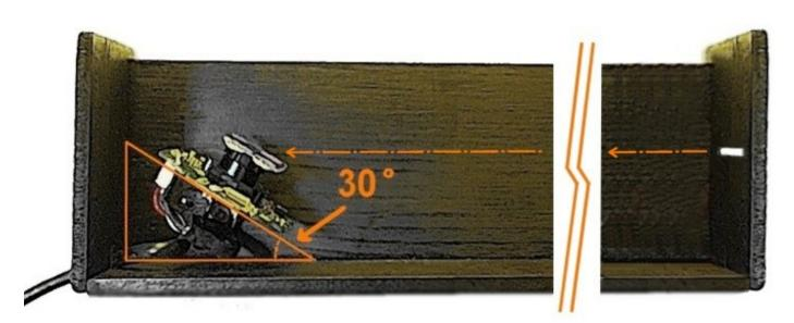
The light entry slit should be horizontal and approximately at the height of the tip of the lens.
