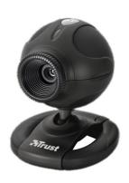
Other essential features are that the lens has a flat, easy-to-remove infrared filter and that the exposure and sensitivity controls are manual and work well. Trusts generally have these characteristics. If the camera is not a WB-6250X, check that the infrared filter can be removed and that it has manual, well-functioning exposure controls, before you change it.
