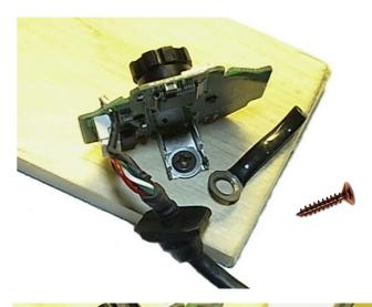
Remove the rubber grommet by cutting it with the wire cutters. (Be careful not to damage the insulation of the cable)
