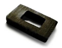
To achieve complete elimination of reflections, the hole should be as narrow and low as possible. Since the height of the lens above the entrance slit can vary from one construction to another, the best way to find its ideal size is to place a strong light behind the slit and test with black cardboard how tight the four walls of the hole can be tightened.
