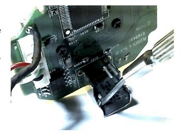
If the button terminals are still attached to the PCB, cut them off at the base using wire cutters or small scissors.
