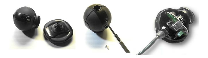
Separate the chamber from the base and unscrew the small screw that holds the two halves of the shell together. Separate the two halves of the shell by pulling hard, without fear, at the end the shell will split and you can extract the printed circuit board.
