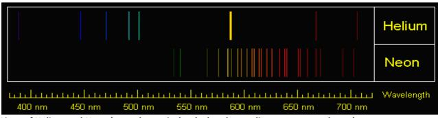
Lines of Helium and Neon (rows theoretical, calculated according to quantum theory)
