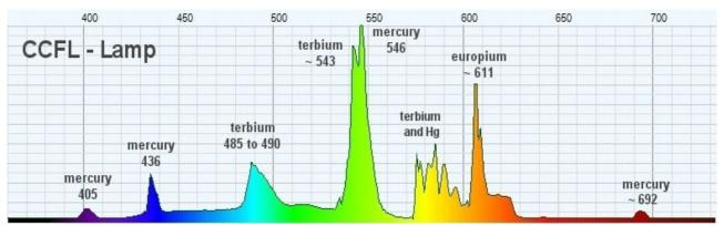
The lines at 436 and 546 nm are accurate. The position of the other rows is not stable and can change from one lamp to another.
