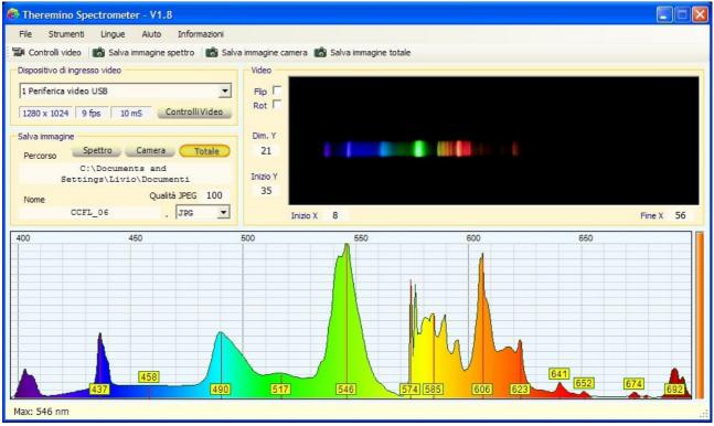
Theremino Spectrometer that displays the spectrum of a fluorescent lamp
