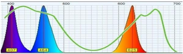
Output of LED ultraviolet, blue, and red superimposed with the photosynthesis efficiency curve
