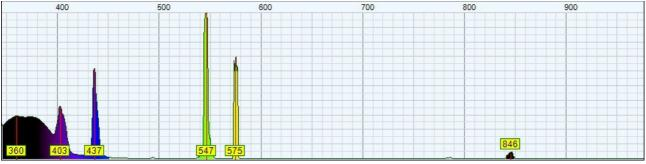
Spectrum of a Philips 15W CLEO tube.
