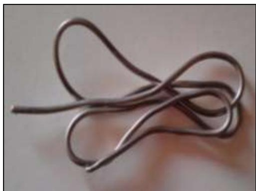
XRF Sample : Soldering Wire
