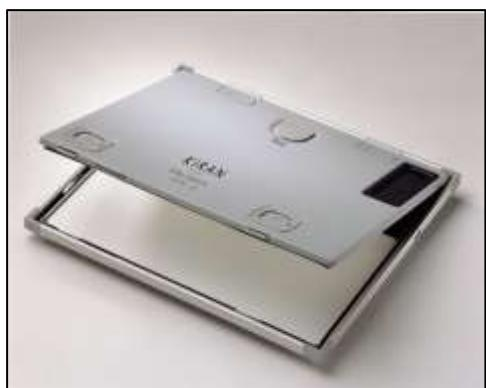
XRF Sample : Intensifying Screen with  $\text{Gd}_2\text{O}_2\text{S}$  and  $\text{LaOBr}$
