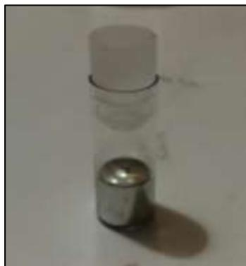
XRF sample: ampoule with mercury
