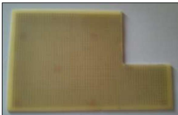
XRF Sample : PCB with Bromine as Flame Retardant
